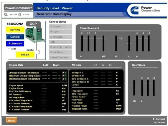
The HMI is a combined industrial PC and 10.4" (264 mm) color touchscreen for monitoring and control of the generator set. The screen is mounted on a console on the front of the GCP2 with gaskets between the touchscreen and the enclosure for environmental protection. It is complete with a real time clock, with separate battery backup and incorporates flash memory.
